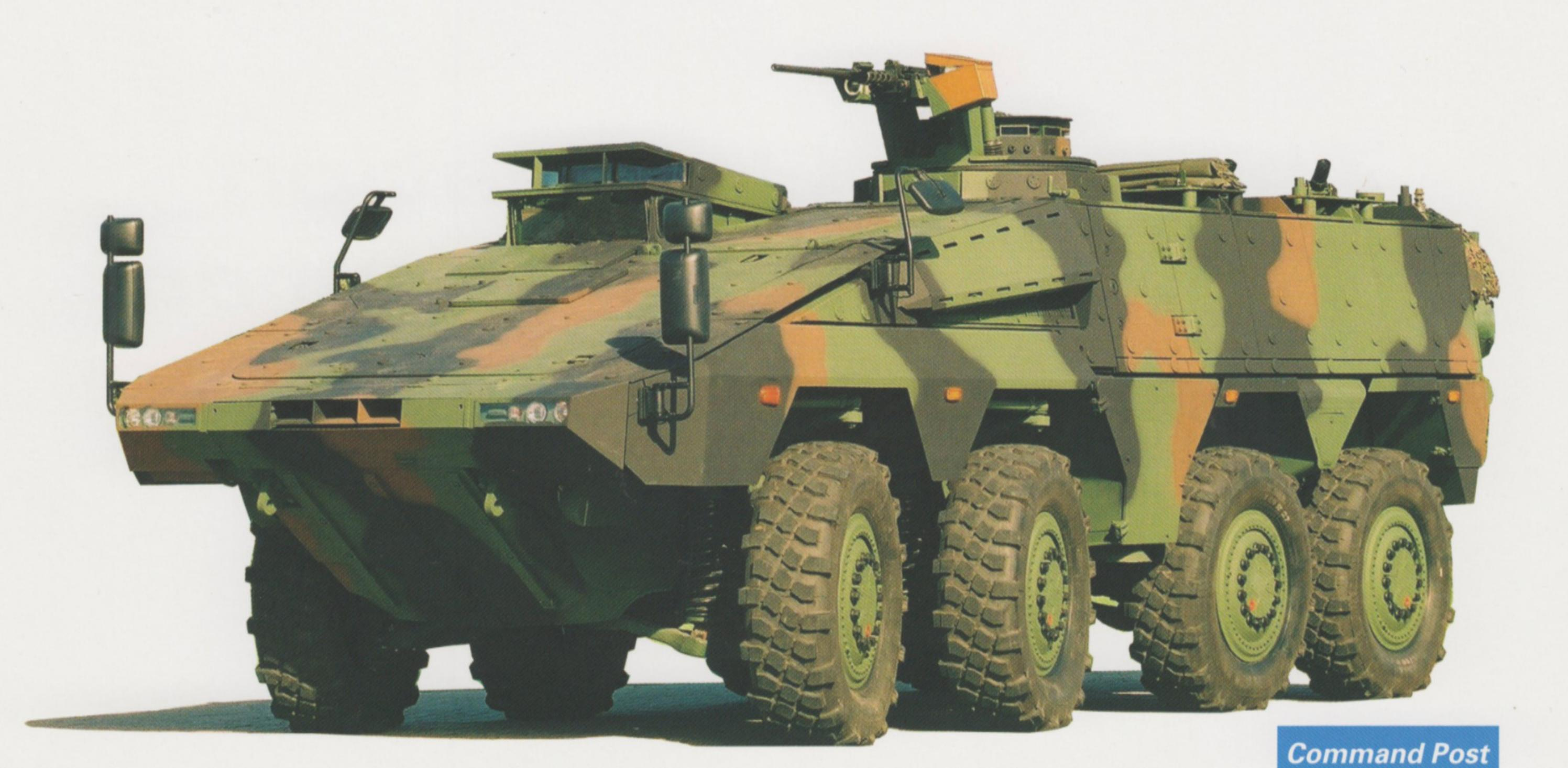
The BOXER 8x8 vehicle is the result of balancing the key military requirements of Protection, Mobility, Payload and ired by the German and Dutch Armies. It has state of the art mine, ballistic and NBC protection in its
